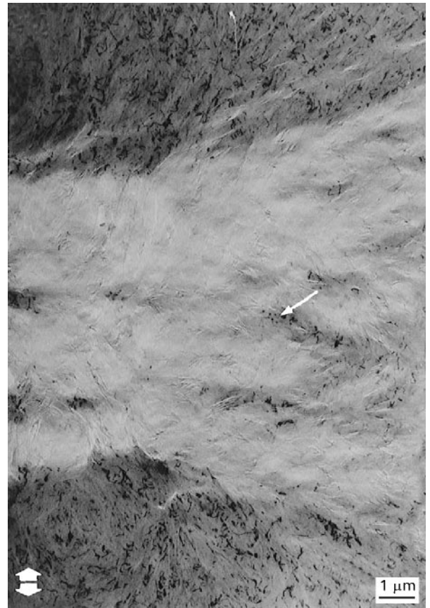
Figure 10 Lower magnification transmission electron micrograph of a deformed equatorial spherulite radius in HMW-HDPE sample E 8:145 drawn to 20% strain. “Islands” of undeformed material are indicated by the small arrows within the intraspherulitic deformation, demonstrating the non-uniform nature of intraspherulitic deformation. The tensile axis is shown by the large arrows.
