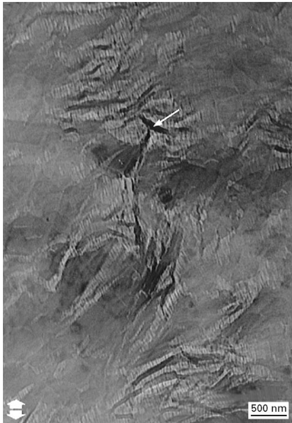
Figure 9 Detail of the intraspherulitic fibrillated regions indicated in Fig. 8. The dark entities that are indicated by the small arrows are possibly lamellae. The tensile axis is shown by the large arrows.
